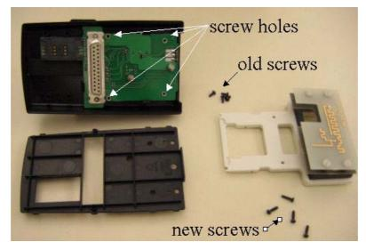
Install the coupler and use the new screws.
