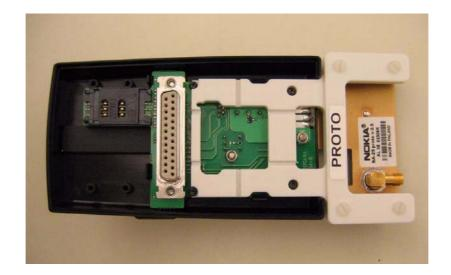
Close the docking station adapter by attaching the bottom plate.
